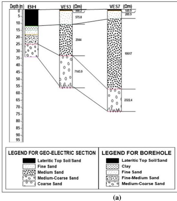
Figure 4a: Correlation of borehole log with VES 3 and VES 7
